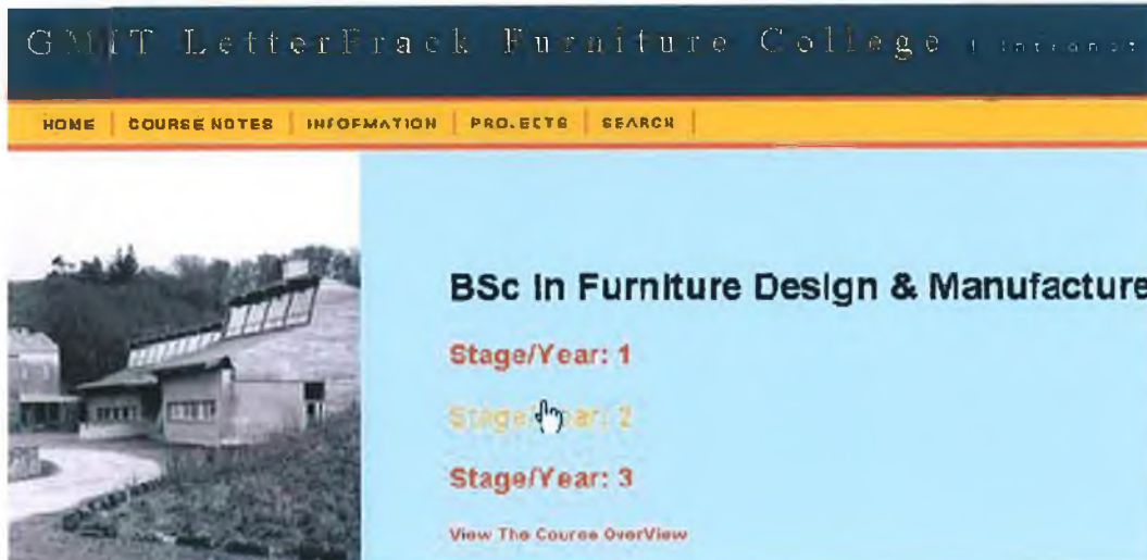
Fig. 24 Once a course is selected links to the stages in that course are displayed. The results displayed are dynamically generated by querying the database to see what stages are available for the selected course. The Course Overview is also displayed dynamically from the database as some courses may not have an overview available.
