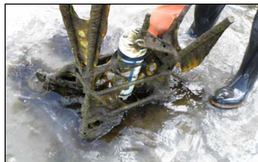
Figure 4.2 – Hydrolab datasonde deployed on site
