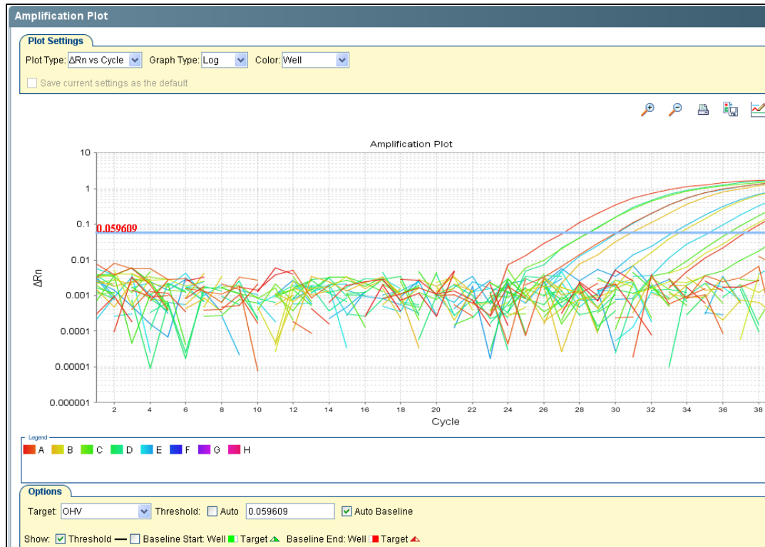
Figure 2.3 – Amplification plot analysed using Applied Biosystems 7500 software to show baseline and threshold of the amplification plots with the threshold set halfway up the exponential phase of the amplification plot.
