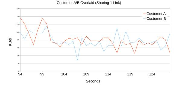
FIGURE 4.9: Customer A and B Sharing one Link
