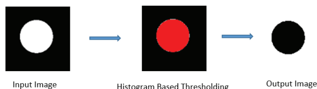
Fig. 2. Detection of a circular object using histogram-based image segmentation.
