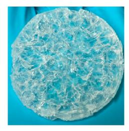
Figure 7. Poor surface quality of FC14 after 72 h of swelling at room temperature.
