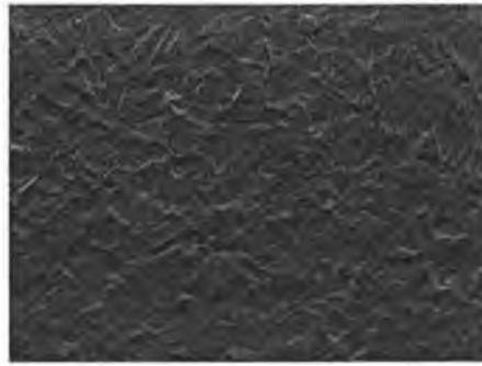
Figure 5.4 – Surface etched by 4 Molar at 360 seconds – 1k magnification (316L)
