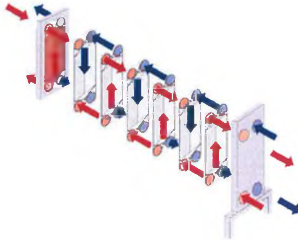
Figure 22 Plate Heat Exchanger source Google.ie
