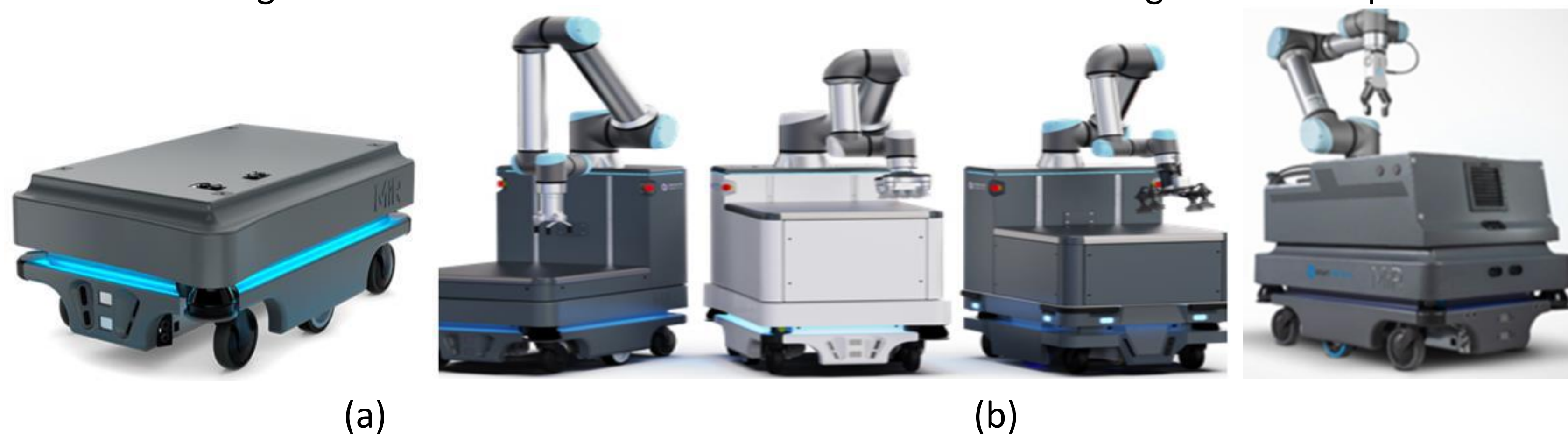
Fig. 1. (a) Autonomous Mobile Robot, (b) Different Combinations of AMR, Robotic Arm Top Modules & Grippers
