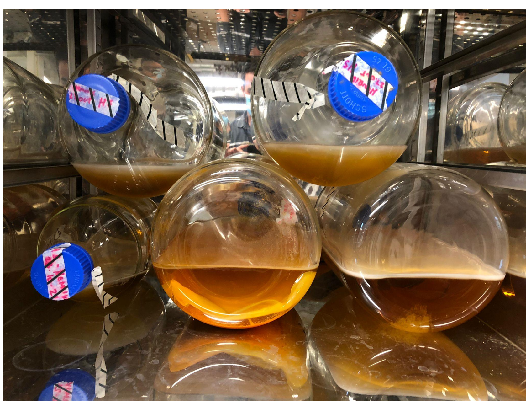
Figure 2. Batches with Komagataeibacter medellinensis in HS medium.
