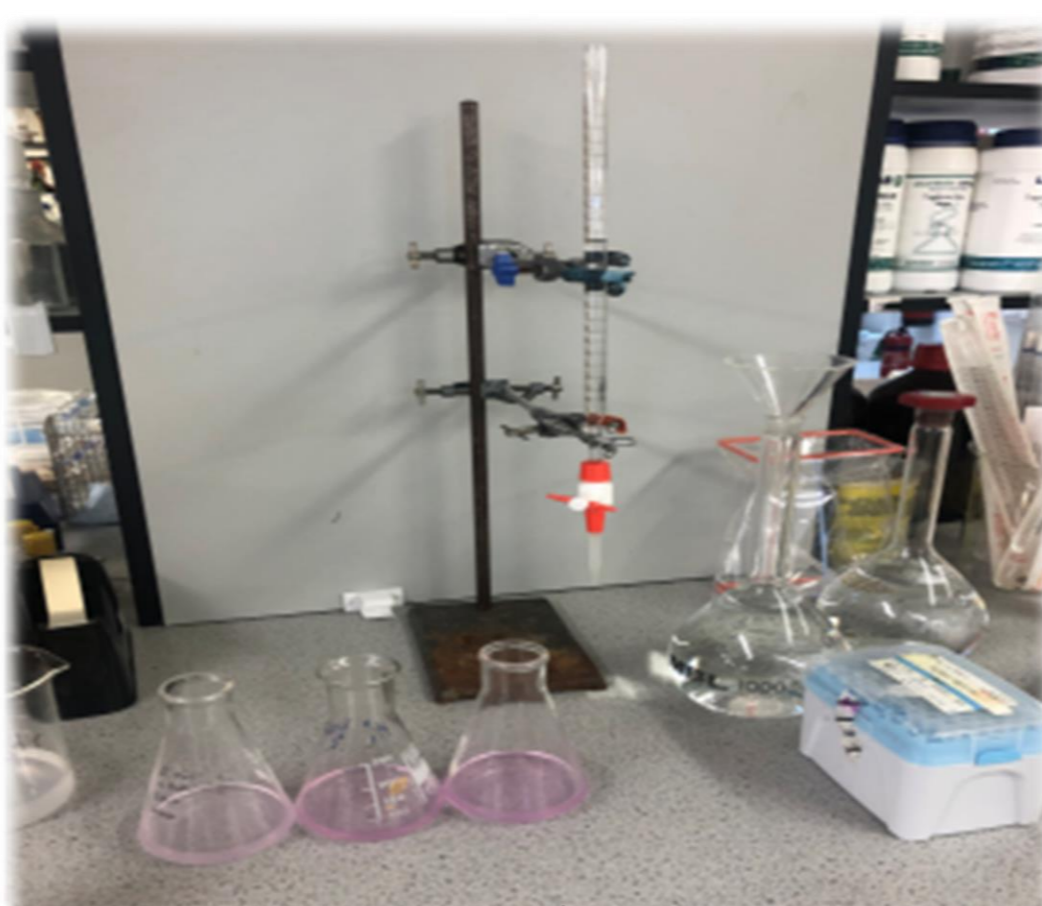
Figure 5 Acid value assay performed in the TUS research hub
