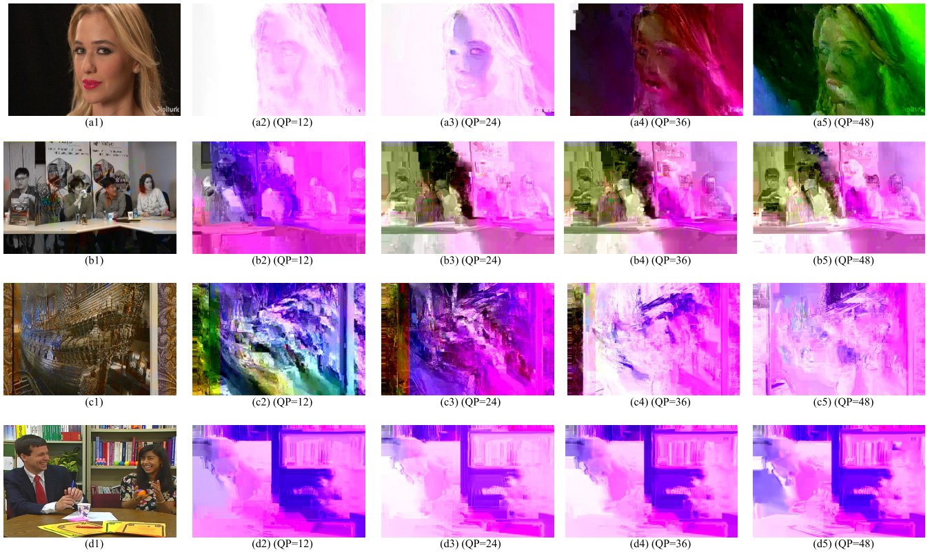
FIGURE 10. Impact of visual distortion of SLEPX at different QP levels with respect to various videos. Parts (a1) – (d1) show frames #07, 29, 19 and 35 of the plain encoded versions of Beauty , Four People , MobCal and Paris video sequences respectively. Parts (a2)-(d2), (a3)-(d3), (a4)-(d4) and, (a5)-(d5) show the encrypted versions of Beauty , Four people , MobCal and Paris video sequences for the indicated QP.
