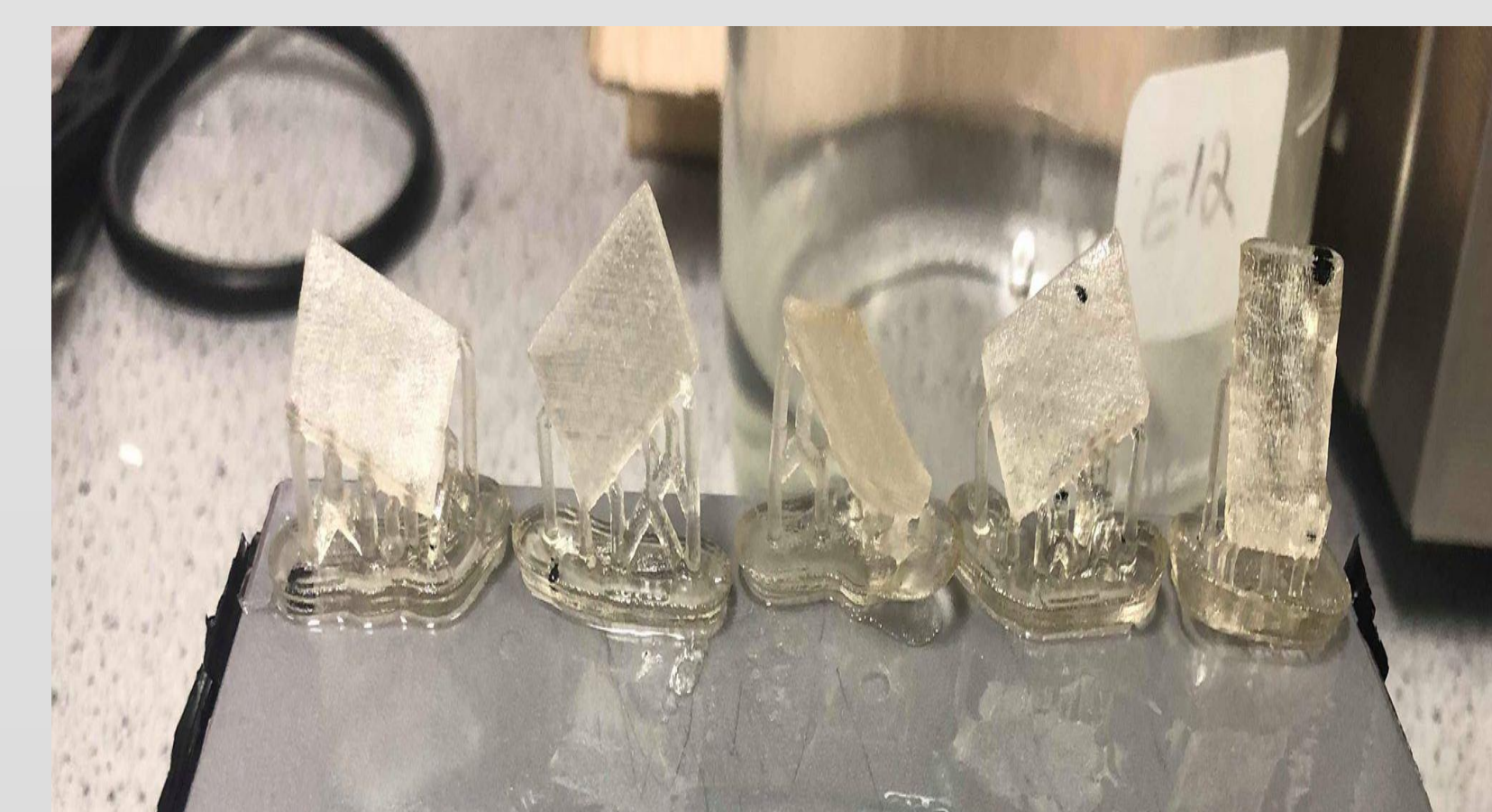
Figure 6: 3D printed tensile bars using novel formulation
