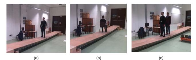
Figure 4. Test scenarios employed – (a) One person standing, (b) One Person and (c) Two Persons standing at midspan of the bridge
