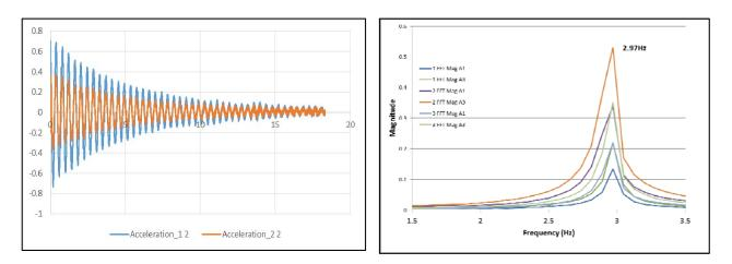
Figure 3. (a) Acceleration response of 8.0m span under self-weight (b) FFT of acceleration traces for 8.0m span under self-weight
