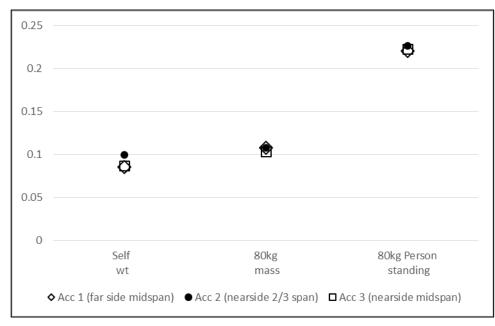
Figure 5. Logarithmic Decrement for Empty Structure and Test Scenarios involving inert mass and humans at midspan.
