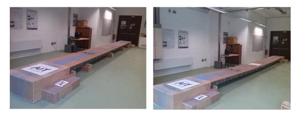
Figure 2. Completed Laboratory Scale FRP Composite Footbridge
