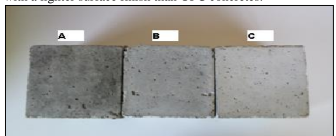
Figure 5: Concrete color variation (A)100% CEM I OPC (B) 20% SCC (C) 50% SCC
