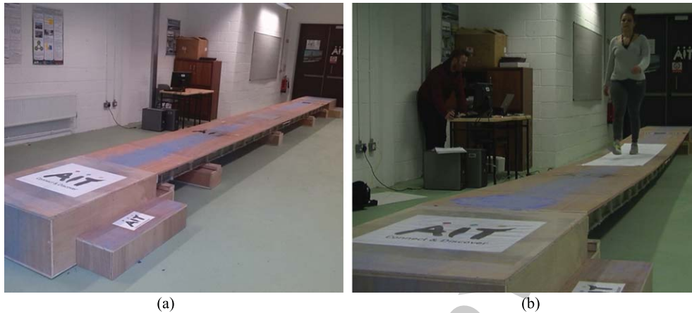
Fig. 3. (a) Laboratory Scale Test Footbridge, (b) Walking trial in progress.
