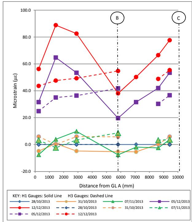
Figure 9. Changes in measured strain along GL 3.5
