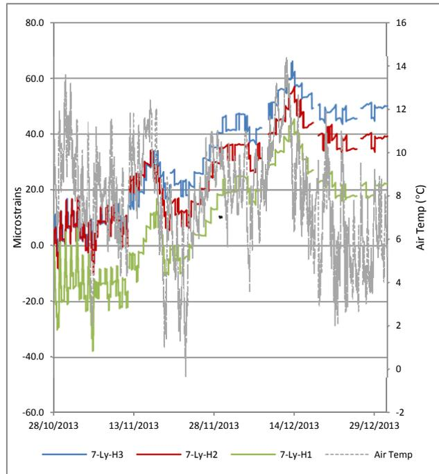
Figure 10. Measured strain (7-Ly) and air temperature
