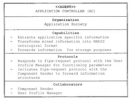
Figure 4.3. The Application Controller agent class diagram
