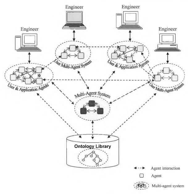
Figure 2.4. High-level view over the architecture of the proposed intelligent collaborative design system
