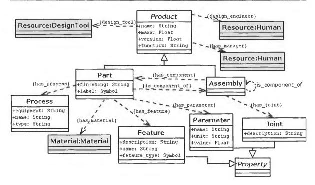
Figure 4.22. UML view over the Structure Ontology
