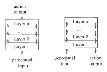
Figure 3.10. Control flow in vertically layered agent architecture (one pass control and two pass control) (Wooldridge 1999)
