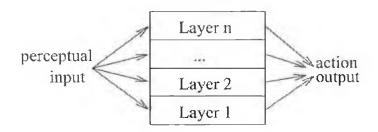
Figure 3.9. Control flow in horizontally layered agent architecture (Wooldridge 1999)
