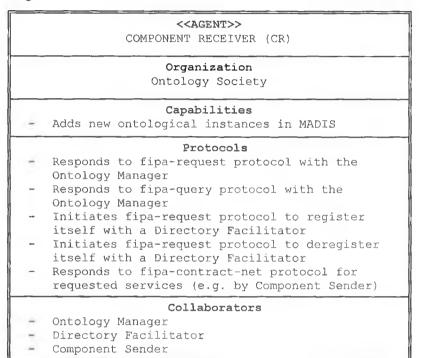
Figure 4.8. The Component Receiver agent class diagram
