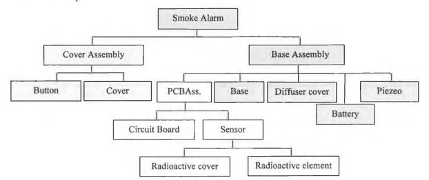
Figure 5.9. The Smoke Alarm structure (Bill of Materials)
