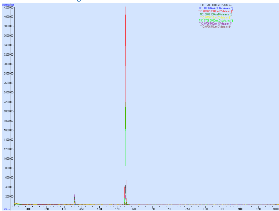
TIC chromatogram from GC-MS of standard curve for sodium butyrate
