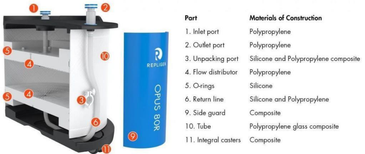
Figure 22: OPUS 80R: Commercial prepacked 80cm in diameter column - cross section (Repligen 2019)
