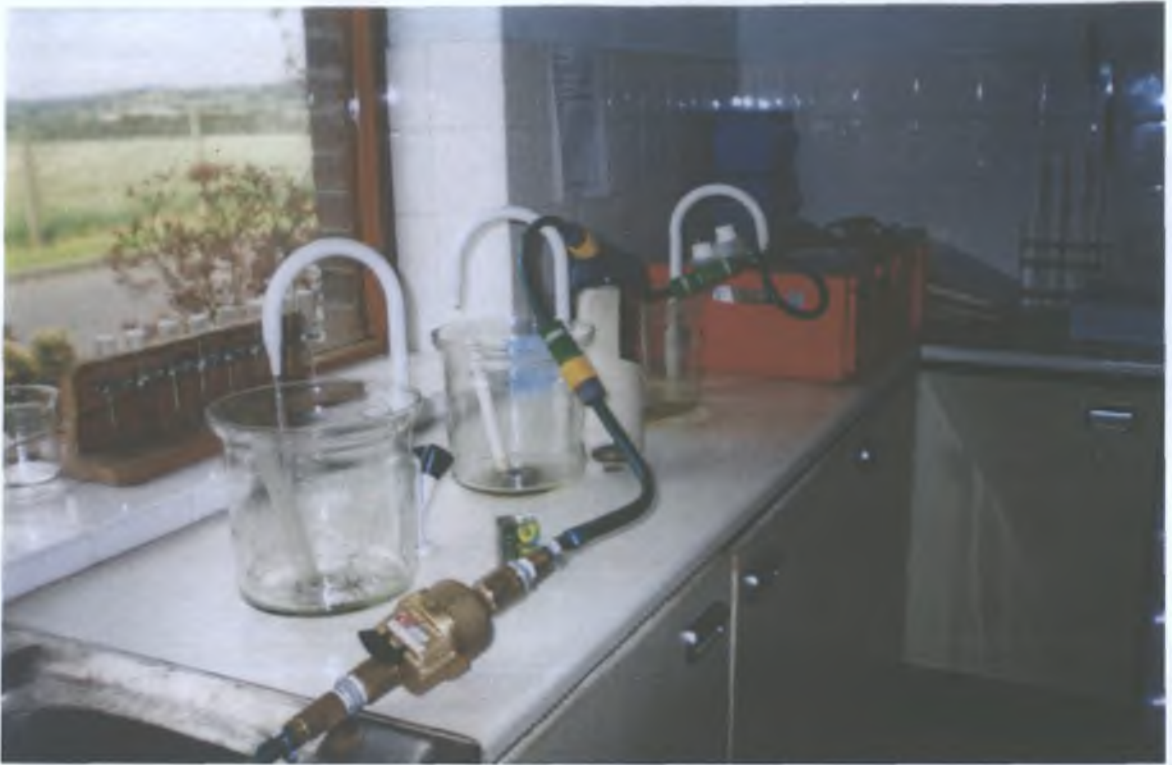
Fig. 3.1 : Cryptosporidium sampling rig in situ in Troyswood Treatment Plant. Picture shows from left to right: Flow restrictor and meter, cartridge housing, Hose connected to Raw Supply Tap.
