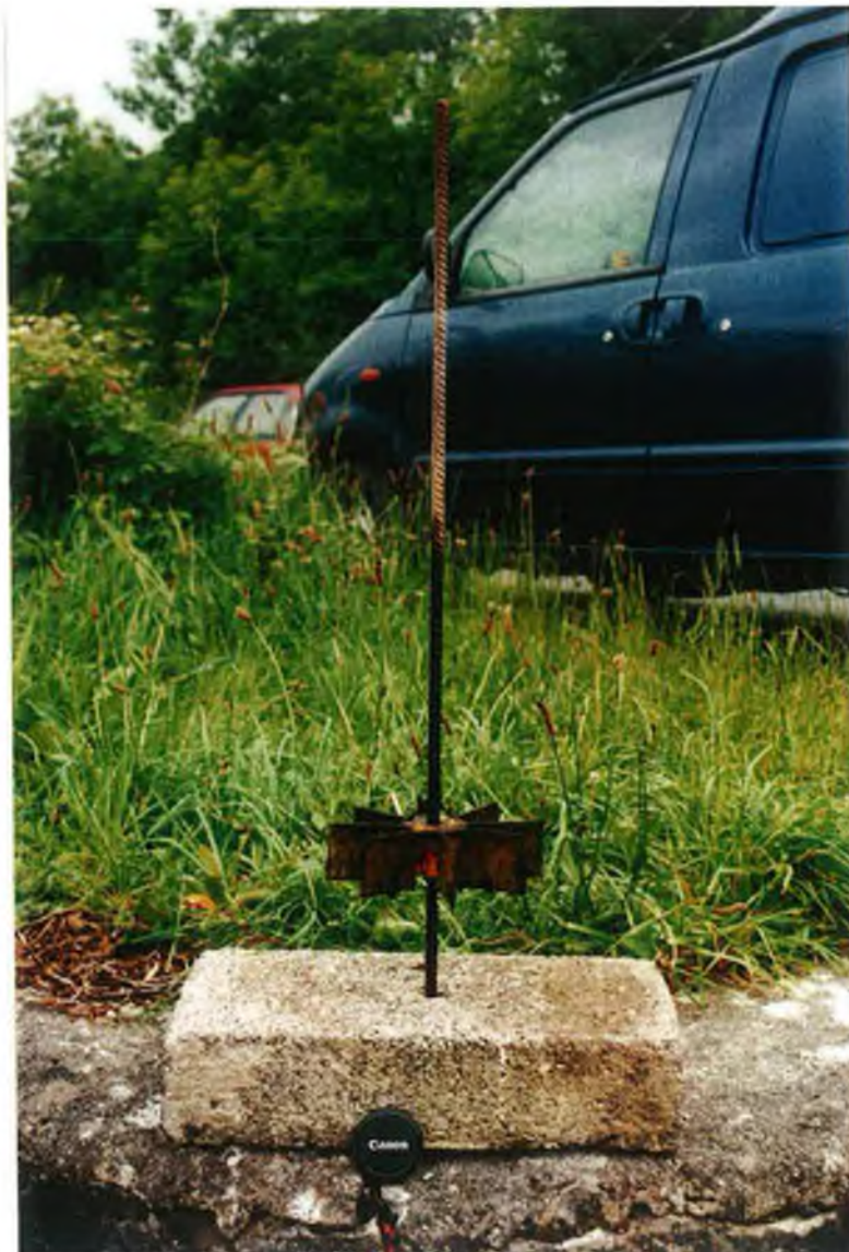
Plate 13: Set-up of glass slides exposed for a one month period at Sriff Bay (site S3) during May 1998. The slides and rubber bung attached to the metal pole. The pole is slotted in to a hole in the concrete block which supports the structure on the bed of the littoral zone. (The camera dust-cap shows scale)
