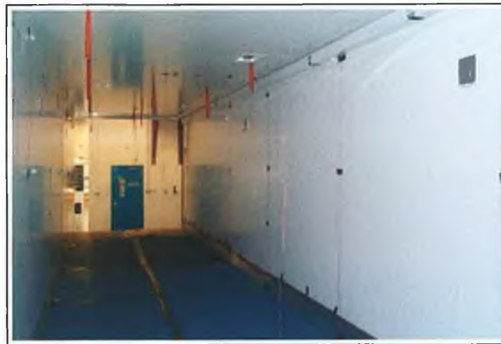
Figure 5.2 Temperature Sensors Distributed within the Trailer Body
