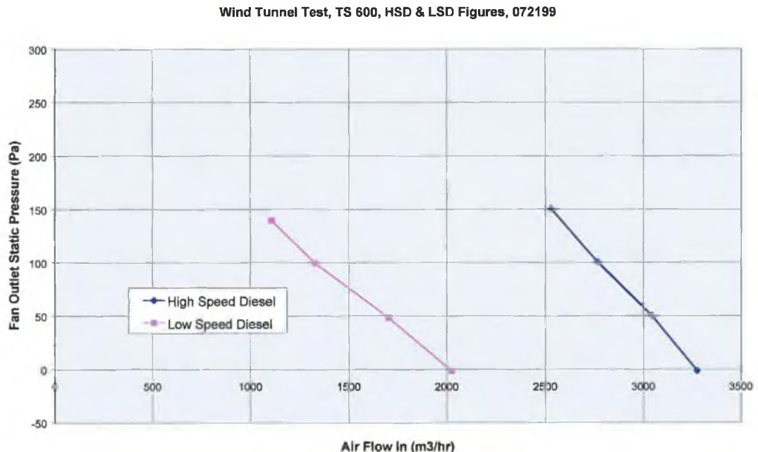
Figure 6.19 Graphical Results of a Wind Tunnel Test carried out on a Truck Unit
