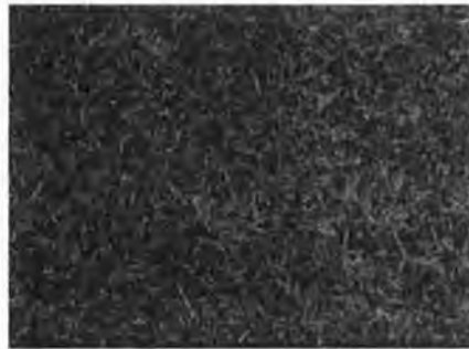
Figure 4.18 Steel with zinc phosphate coating applied under laboratory conditions
