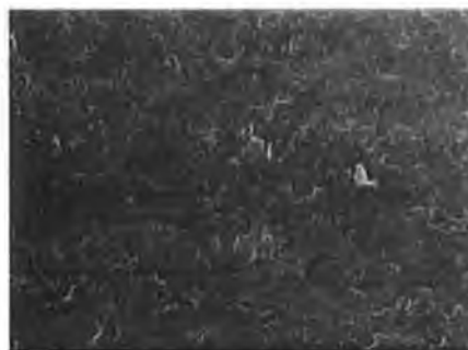
Figure 4.17 Steel with iron phosphate coating applied under laboratory conditions
