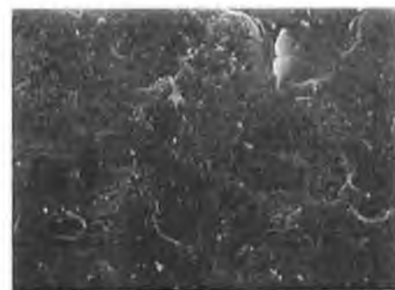
Figure 4.17 Steel with iron phosphate coating applied under laboratory conditions
