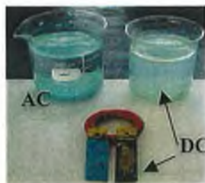
Figure 4.8 Photograph of brass electrodes and solutions after AC and DC power
