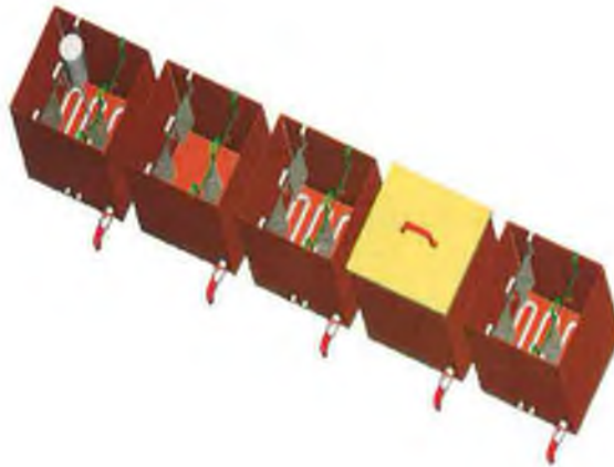
Figure 5.5 Assembly 3D model of pilot plant
