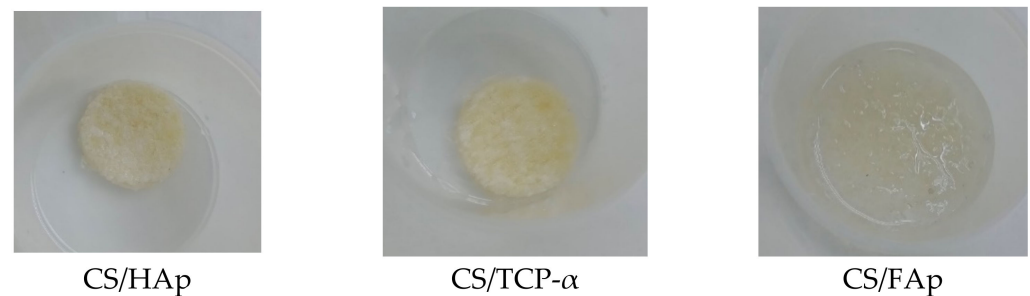
Figure 8. The scaffolds' physical condition following submerging in SBF for two weeks, where the swelling of chitosan was observed the most in CS/FAp.
