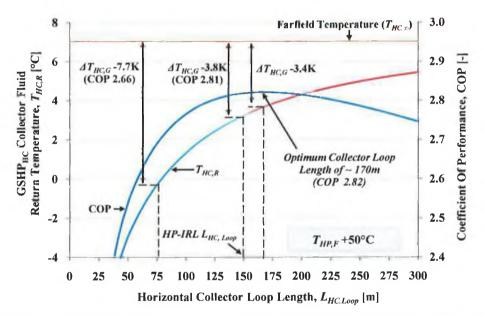
FIGURE 5.3 VARIATION IN THE COLLECTOR FLUID RETURN TEMPERATURE AND RESULTING COP WITH COLLECTOR LENGTH FOR +50°C OUTPUT TEMPERATURE.
