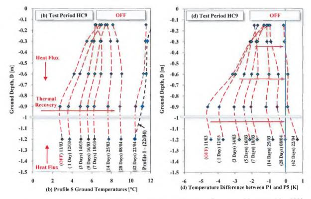
FIGURE 4.32 LONG-TERM RETRACTION OF THE THERMALLY AFFECTED ZONE FROM MARCH TO MAY 2009 SUBSEQUENT TO THE CESSATION OF TEST PERIOD HC9.
