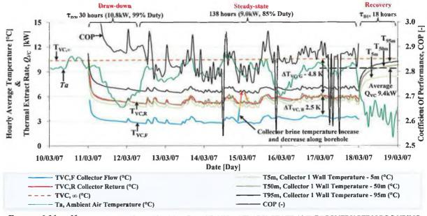
FIGURE 6.11 HOURLY AVERAGED THERMAL DRAWDOWN, STEADY-STATE AND RECOVERY PERIODS DURING TEST PERIOD VC1.
