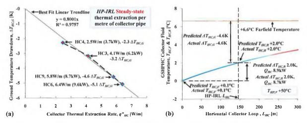
**FIGURE 5.2** (A) GROUND TEMPERATURE DRAWDOWN ( $\Delta T_{HC,G}$ ) VERSUS COLLECTOR THERMAL EXTRACTION RATE PER METER OF COLLECTOR PIPE (1500m) RECORDED UNDER STEADY-STATE THERMAL EXTRACTION CONDITION IN TEST PERIODS HC3, HC4, HC6 AND HC9 AND (B) LONG-TERM STEADY STATE PREDICTED VARIATION TO THE COLLECTOR FLUID TEMPERATURE ALONG THE COLLECTOR LENGTH WHEN EXPOSED TO A UNIFORM FARFIELD GROUND TEMPERATURE OF +6.6°C VERSUS TEMPERATURES RECORDED IN TEST PERIOD HC9.
