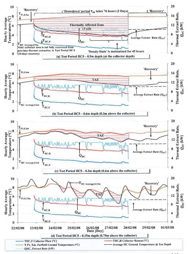
**FIGURE 4.27** TEST PERIOD HC5 THERMAL DEGRADATION OF COLLECTOR AREA AT DEPTHS BETWEEN 0.15M AND 0.9M.
