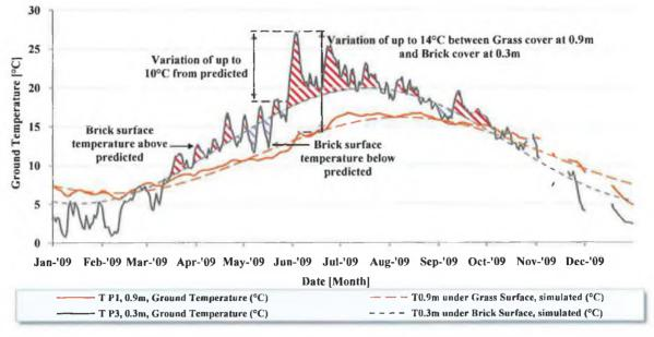
FIGURE 5.6 DAILY AVERAGED MEASURED AND PREDICTED GROUND TEMPERATURES UNDER A GRASS AND BRICK COVERED SURFACE AT DEPTHS OF 0.3M AND 0.9M DURING 2009.
