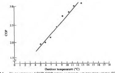
FIGURE 2.14 VARIATION IN ASHP COP WITH AMBIENT AIR TEMPERATURE (KENT, 1997).
