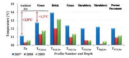
FIGURE 4.39 ANNUAL AVERAGED GROUND SURFACE TEMPERATURES AT 0.3M DEPTH.
