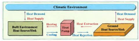
FIGURE 1.5 INTERDEPENDENCE BETWEEN BUILDING DEMAND, CLIMATE AND HEAT SOURCE/SINK.
