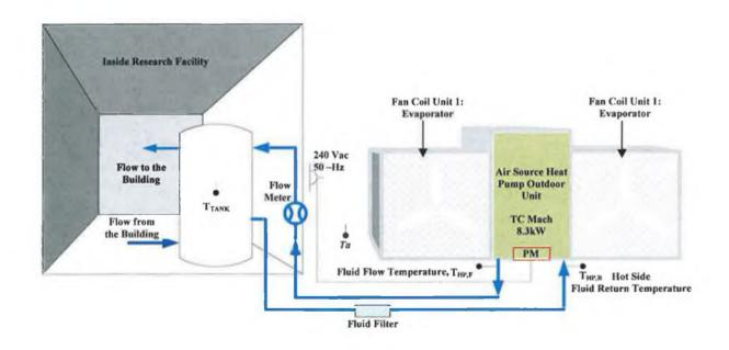
$\label{eq:Figure 3.26} Figure 3.26 \qquad \mbox{Configuration of the ASHP} \ \mbox{and measurement instrumentation}.$
