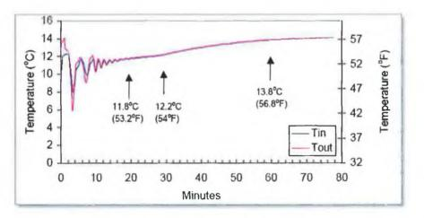
**FIGURE 6.4** VERTICAL COLLECTOR FARFIELD GROUND TEMPERATURE IN LULEÅ SWEDEN (GEHLIN, 2002).
