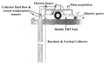
FIGURE 2.10 APPARATUS USED TO CONDUCT A THERMAL RESPONSE TEST (GEHLIN, 2002).
