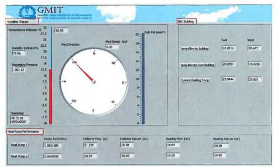
FIGURE 3.28 LABVIEW FRONT PANEL CREATED TO DISPLAY SUMMARY DATA FROM THE WEATHER STATION, THE IIBC AND BOTH GSHPS.
