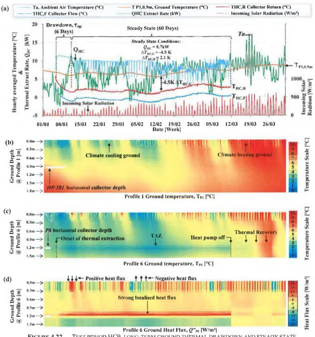
FIGURE 4.22 TEST PERIOD HC9, LONG-TERM GROUND THERMAL DRAWDOWN AND STEADY STATE EXTRACTION (A) CLIMATE AND GROUND TEMPERATURE, (B) 3-D TEMPERATURE MAP IN REFERENCE PROFILE 1, (C) 3-D TEMPERATURE MAP IN COLLECTOR REGION SHOWING TAZ AND (D) 3-D HEAT FLUX MAP WITH POSITIVE DOWNWARD HEAT FLUX IN RED, NEGATIVE UPWARD HEAT FLUX IN BLUE.
