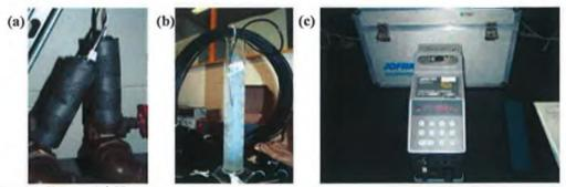
**FIGURE F.2** (A) HEAT PUMP COLLECTOR FLOW AND RETURN TEMPERATURE SENSORS IN SITU, (B) TEMPERATURE SENSOR ICE BATH CALIBRATION AND (C) *ZOFRA* TEMPERATURE SENSOR CALIBRATOR.
