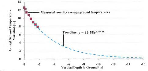
**FIGURE 6.1** EXTRAPOLATION OF MEASURED MONTHLY AVERAGED DATA TO PREDICT GROUND TEMPERATURE VARIATION FROM MEAN TO A DEPTH OF 16M IN GALWAY.
