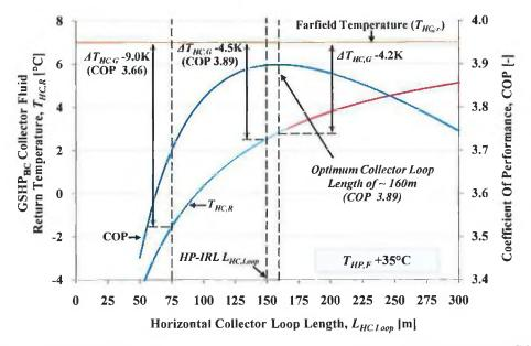
FIGURE 5.4 VARIATION IN THE COLLECTOR FLUID RETURN TEMPERATURE AND RESULTING COP WITH COLLECTOR LENGTH FOR +35°C OUTPUT TEMPERATURE.
