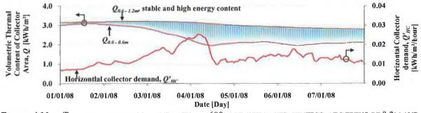
FIGURE 4.11 THERMAL ENERGY CONTENT WITHIN A 600MM THICK LAYER CENTRED AT DEPTHS OF 0.3M AND 0.9M IN PROFILE 1 VERSUS A PROJECTED COLLECTOR THERMAL DEMAND AT PEAK HEATING SEASON, JANUARY, 2008.
