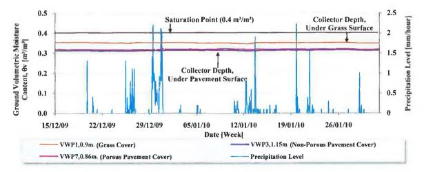
FIGURE 4.8 RECORDED RAINFALL AND HOURLY AVERAGED GROUND VOLUMETRIC MOISTURE CONTENT AT COLLECTOR DEPTH (DECEMBER 2009 TO JANUARY 2010).
