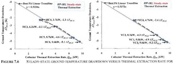
THE (A) HORIZONTAL COLLECTOR AND (B) VERTICAL COLLECTOR.
