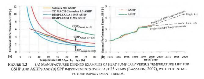
The efficiency of a heat pump over a heating season is referred to as the Seasonal Performance Factor (SPF), details of which are provided in Appendix A. Figure 1.3(b) highlights that there has been a steady increase in the SPF of both ASHP and GSHP systems over the past 30 years, with recent (2000) values 60% above those in 1976. Projecting past performance trends forward to 2020 indicate that SPFs ranging between 3.5 and 4.3 should be possible.
