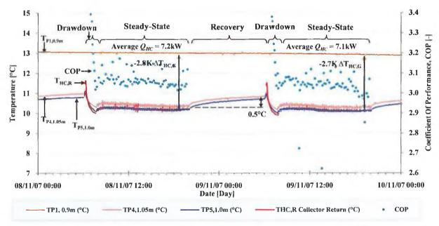
**FIGURE 4.34** DRAWDOWN AND RECOVERY OF THE GROUND TEMPERATURE IN THE GSHP<sub>HC</sub> COLLECTOR REGION DURING NOVEMBER, 2007 (HC3).
