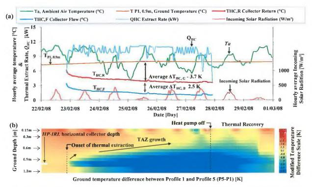
FIGURE 4.26 (A) SHORT-TERM, INTENSIVE THERMAL EXTRACTION (93%) DURING TEST PERIOD HC5 AND (B) 3-D TEMPERATURE DIFFERENCE MAP ILLUSTRATING THE TAZ AROUND THE HORIZONTAL COLLECTOR DURING TEST HC8, ESTABLISHED BY SUBTRACTING GROUND TEMPERATURES AT PROFILE 1 FROM GROUND TEMPERATURES AT PROFILE 5 (P5-P1).
