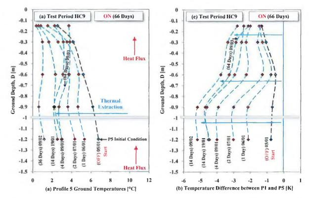
FIGURE 4.31 LONG-TERM EXPANSION OF THE THERMALLY AFFECTED ZONE FROM JANUARY TO MARCH 2009 DURING TEST PERIOD HC9.
