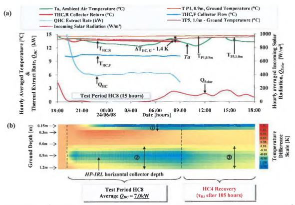
**FIGURE 4.25** (A) SHORT-TERM, MODERATE THERMAL EXTRACTION FROM HORIZONTAL COLLECTOR AND (B) TAZ AROUND THE HORIZONTAL COLLECTOR DURING TEST HC8 ESTABLISHED BY SUBTRACTING GROUND TEMPERATURES AT PROFILE 1 FROM GROUND TEMPERATURES AT PROFILE 5 (P5-P1).
