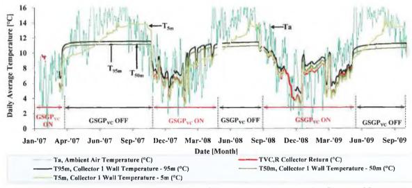
FIGURE 6.2 VERTICAL COLLECTOR (BOREHOLE 1) WALL TEMPERATURES AT 5M, 50M AND 95M BETWEEN 2007 AND 2009.
