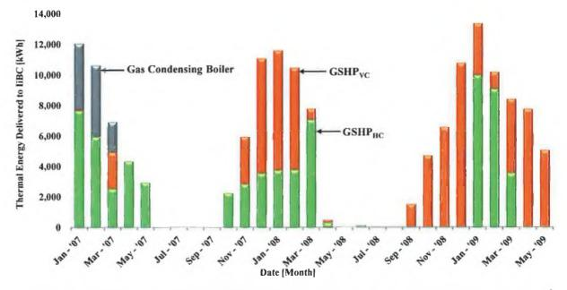
**FIGURE 3.4** RESPECTIVE CONTRIBUTIONS OF THE GSHP<sub>HC</sub>, GSHP<sub>VC</sub> & GAS HEATING SYSTEMS TO THE IIBC HEAT DEMAND PER MONTH BETWEEN JANUARY, 2007 AND JUNE, 2009.
