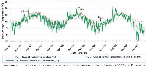
**FIGURE 7.1** HEAT PUMP SOURCE TEMPERATURE COMPARISON BETWEEN JANUARY 2007 AND FEBRUARY 2010.
