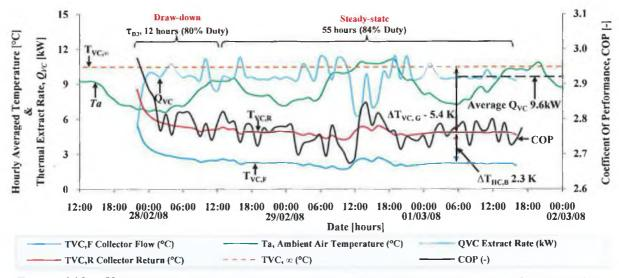
FIGURE 6.10 HOURLY AVERAGED THERMAL DRAWDOWN AND STEADY-STATE PERFORMANCE DURING TEST PERIOD VC3.
