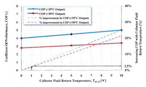
FIGURE 4.18 PERCENTAGE IMPROVEMENT IN *HP-IRL* COP WITH INCREASED COLLECTOR FLUID RETURN TEMPERATURE.
