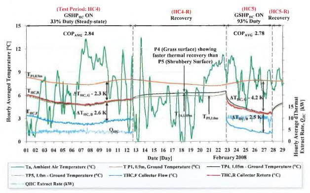
FIGURE 4.35 DRAWDOWN AND RECOVERY OF THE GROUND TEMPERATURE IN THE COLLECTOR REGION OF THE GSHP<sub>HC</sub> DURING TEST PERIODS HC4 AND HC5.
