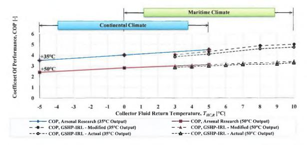
**FIGURE 4.17** COMPARISON OF HEAT PUMP PERFORMANCE AS MEASURED USING INTERNATIONAL STANDARD EN-14511 AND DATA FROM *HP-IRL* STUDY.
