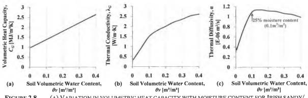
FIGURE 2.8 (A) VARIATION IN VOLUMETRIC HEAT CAPACITY WITH MOISTURE CONTENT FOR IRISH SANDY/ SILTY LOAM SOIL WITH AN AVERAGE BULK DENSITY OF 1200KG/M<sup>3</sup> (B) VARIATION OF SOIL THERMAL CONDUCTIVITY, AND (C) VARIATION OF THERMAL DIFFUSIVITY (WITH INCREASED IN SOIL MOISTURE CONTENT FOR IRISH SANDY LOAM SOIL WITH AN AVERAGE BULK DENSITY OF 1200KG/M<sup>3</sup>) (LOHAN *ET AL.*, 2006).
