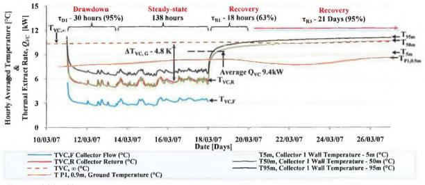
**FIGURE 6.14** HOURLY AVERAGED BOREHOLE THERMAL DRAWDOWN, STEADY-STATE AND RECOVERY AFTER INTENSIVE TEST PERIOD VC1.
