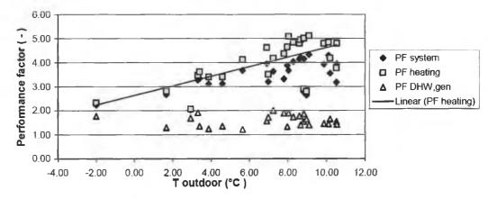
FIGURE 2.17 ASHP PERFORMANCE DATA AS A FUNCTION OF EXTERNAL AMBIENT AIR TEMPERATURE IN 2006/2007 (VERHELST *ET AL.*, 2008).
