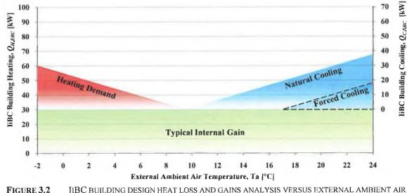
FIGURE 3.2 IIBC BUILDING DESIGN HEAT LOSS AND GAINS ANALYSIS VERSUS EXTERNAL AMBIENT AIR TEMPERATURE.
