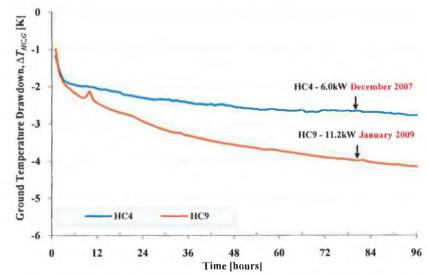
FIGURE 4.20 HOURLY AVERAGED GROUND TEMPERATURE DRAWDOWN FOR TEST PERIODS HC4 AND HC9.
