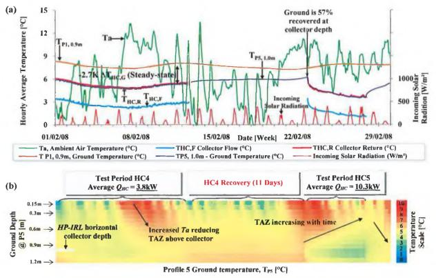
FIGURE 4.29 (A) GROUND THERMAL EXTRACTION AND RECOVERY FOR TEST PERIODS HC4 AND HC5 AND (B) 3-D TRANSIENT TEMPERATURE MAP AT PROFILE 5.
