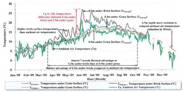
FIGURE 5.5 VARIATIONS IN THE GROUND TEMPERATURE UNDER BRICK AND GRASS SURFACE COVERS DURING 2009.
