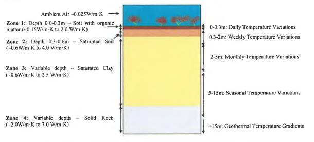
FIGURE 2.7 GROUND TEMPERATURE AND CONDUCTIVITY VARIATIONS WITH DEPTH.
