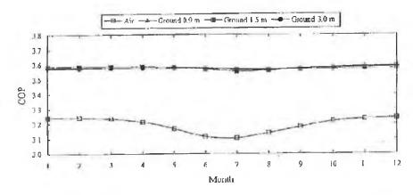
FIGURE 2.16 PREDICTED MONTHLY HEATING COPS FOR AIR AND GROUND SOURCE HEAT PUMP SYSTEMS (DE SWARDT AND MEYER, 2001).
