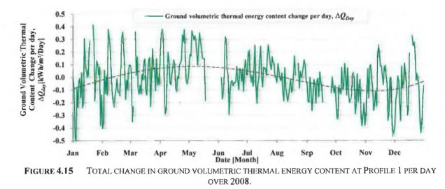
While it is evident from Figure 4.15 that the ground thermal energy provision increases and decreases with the seasons, there is a substantial variation in the ground thermal content from day to day and potential exists to operate a suitable collector to take advantage of the peaks and use the thermal storage to avoid the troughs. This concept is explored further in Section 5.2.
