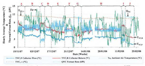
FIGURE 6.16 LONG-TERM VARIABLE THERMAL EXTRACTION DURING TEST PERIOD VC2.
