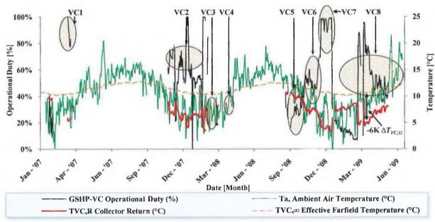
FIGURE 6.7 TIMING OF THE EIGHT GSHP<sub>VC</sub> TEST PERIODS (2007-2009) AND CORRESPONDING DUTY.
