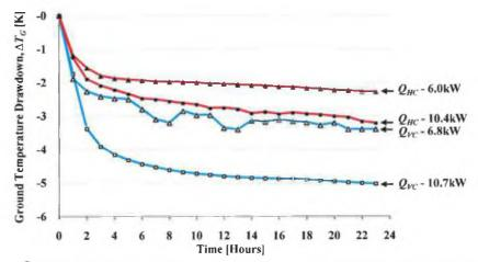
**FIGURE 7.5** COMPARING THE DRAWDOWN OF THE GROUND TEMPERATURE IN THE VICINITY OF BOTH THE HORIZONTAL COLLECTOR ( $\Delta T_{HC, G}$ ) AND THE VERTICAL COLLECTOR ( $\Delta T_{HC, G}$ ) VERSUS EXTRACT RATES (Q), RESULTS WERE OBTAINED FROM TESTS CARRIED OUT ON VARIOUS DATES IN 2007.
