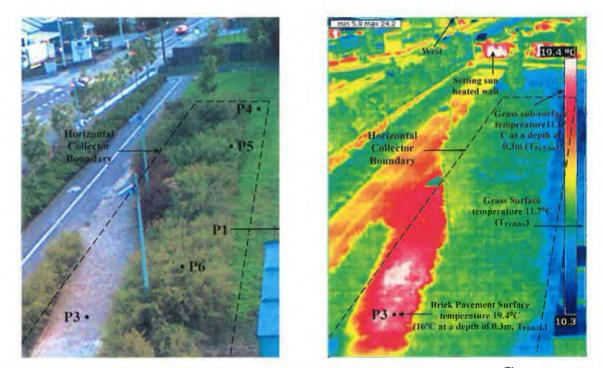
FIGURE 4.37 THERMAL IMAGE OF HORIZONTAL COLLECTOR SURFACE, AT 10PM ON THE 18<sup>TH</sup> OF APRIL 2009.
