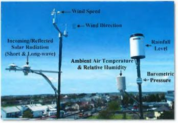
FIGURE 3.9 IIBC'S ROOF MOUNTED, AUTOMATED WEATHER STATION INSTALLED IN 2006.
