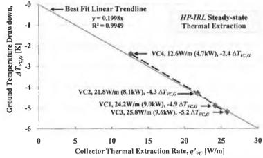
**FIGURE 6.12** GROUND TEMPERATURE DRAWDOWN ( $\Delta T_{VC,G}$ ) RECORDED UNDER STEADY-STATE THERMAL EXTRACTION CONDITIONS DURING TEST PERIODS VC1, 2, 3 AND 4.
