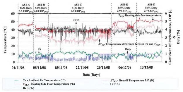
FIGURE 6.21 HOURLY AVERAGED ASHP PERFORMANCE CHARACTERISTICS DURING TEST PERIOD AS1.
