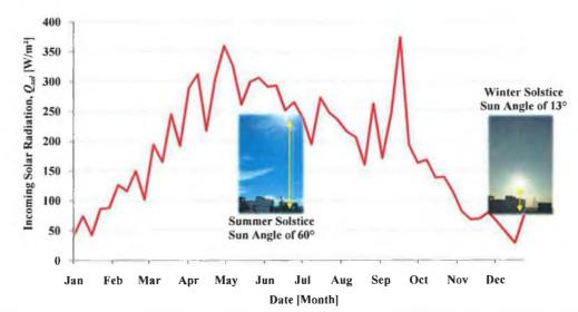
**FIGURE 3.11** INCOMING WEEKLY AVERAGED GLOBAL SOLAR RADIATION RECORDED BY *HP-IRL* WEATHER STATION DURING 2008.
