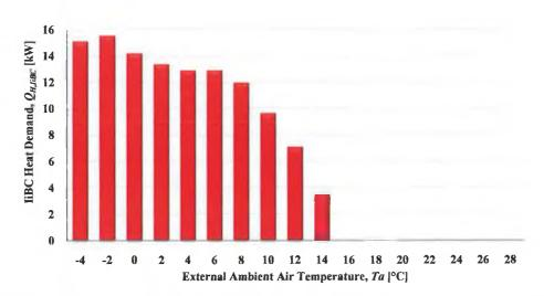
**FIGURE 3.5** TOTAL HEAT DEMAND OF THE IIBC FROM THE HEAT PUMPS AS A FUNCTION OF EXTERNAL AMBIENT AIR REQUIREMENTS.
