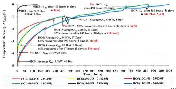
**FIGURE 4.24** THERMAL RECOVERY OF THE COLLECTOR REGION WITHIN PROFILE 5 AFTER TEST PERIODS HC4 THROUGH HC9.
