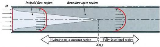
FIGURE K.1 LAMINAR, HYDRODYNAMIC BOUNDARY LAYER DEVELOPMENT IN THE COLLECTOR PIPE.
