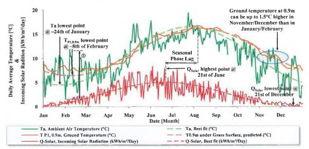
FIGURE 4.2 PROFILE OF DAILY AVERAGED SOLAR RADIATION, AMBIENT AIR TEMPERATURE AND GROUND TEMPERATURE AT 0.9M DURING 2008 VERSUS THAT PREDICTED BY EQUATION 2.1.
