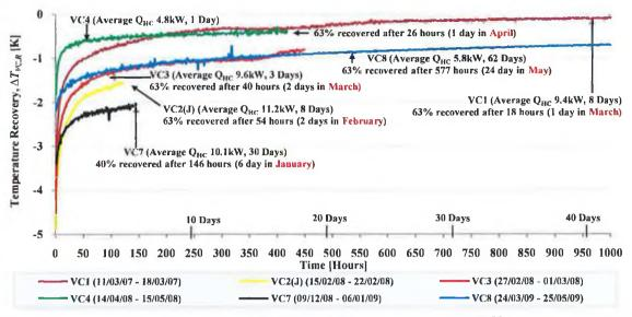
FIGURE 6.13 THERMAL RECOVERY OF THE VERTICAL COLLECTOR AT A DEPTH OF 50M AFTER TEST PERIODS VC1 TO VC8.
