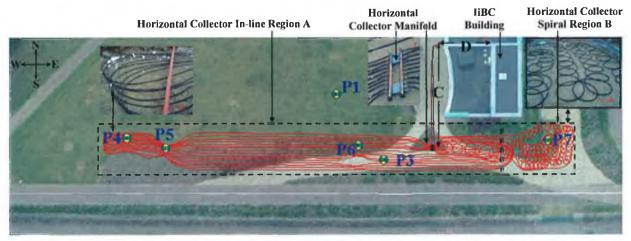
**FIGURE 3.16** AERIAL PHOTOGRAPH OF HORIZONTAL COLLECTOR REGION, UPON WHICH THE ACTUAL COLLECTOR CONFIGURATION HAS BEEN SUPERIMPOSED FROM PHOTOS TAKEN DURING INSTALLATION.
