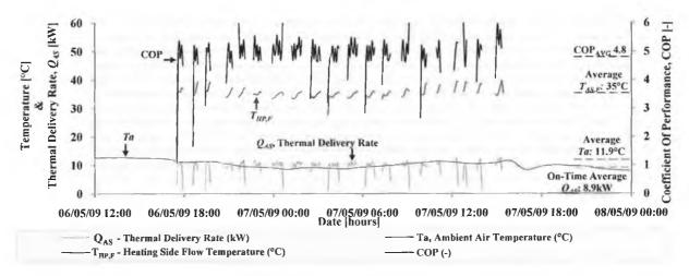
**FIGURE 6.26** FIVE MINUTE RECORDING INTERVAL OF THE ASHP PERFORMANCE CHARACTERISTICS DURING TEST PERIOD AS5 WITH +35°C HEAT PUMP FLOW TEMPERATURE ( $T_{HP,F}$ ).
