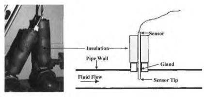
FIGURE 3.15 TEMPERATURE SENSOR IN SITU.
