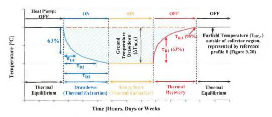
**FIGURE 4.19** SCHEMATIC OF THERMAL EXTRACTION AND RECOVERY CHARACTERISTICS, TO DEFINE DRAWDOWN, STEADY-STATE AND RECOVERY PERIODS ASSOCIATED WITH HEAT PUMP COLLECTOR OPERATION.
