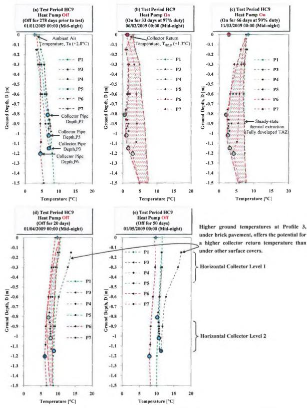
FIGURE 4.30 LONG-TERM EXPANSION AND CONTRACTION OF THE THERMALLY AFFECTED ZONE FROM TEST PERIOD HC9.
