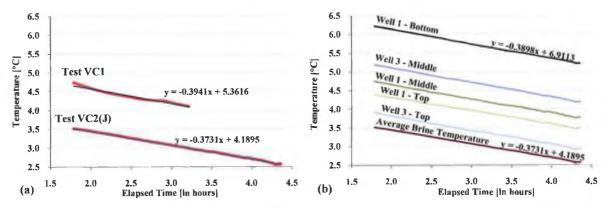
FIGURE 6.19 NATURAL LOG PROGRESSION OF THERMAL EXTRACTION FOR (A) TWO TIME PERIODS VC1 AND VC2(J) AND (B) COLLECTOR WALL TEMPERATURES DURING TEST PERIOD VC2(J).
