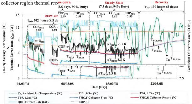
FIGURE 4.21 HOURLY AVERAGED THERMAL DRAWDOWN, STEADY-STATE AND RECOVERY FOR TEST PERIOD HC6.
