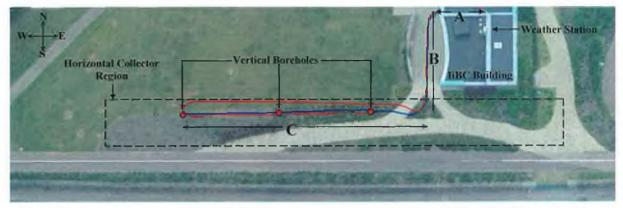
**FIGURE 3.23** AERIAL PHOTOGRAPH SHOWING LOCATIONS OF THE THREE VERTICAL COLLECTOR BOREHOLES RELATIVE TO EACH OTHER, THE HORIZONTAL COLLECTOR AND THE IIBC BUILDING.
