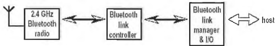
Figure 2.9 Functional blocks in a Bluetooth system [Bluetooth 2001].
