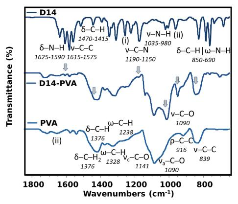
Figure A3. Detailed FTIR spectra of pure D14, PVA and the conjugated D14.
