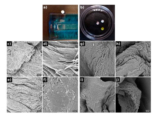
**Figure 1.** Macroscopic images of the PVA spheres (**a**,**b**) and its morphology evaluated by SEM from the surface (**c**,**e**,**g**,**i**) and internal (**d**,**f**,**h**,**j**) structure of (**c**,**d**) pure PVA, (**e**,**f**) doxo-PVA, (**g**,**h**) D14-PVA, (**i**,**j**) D14-doxo-PVA.
