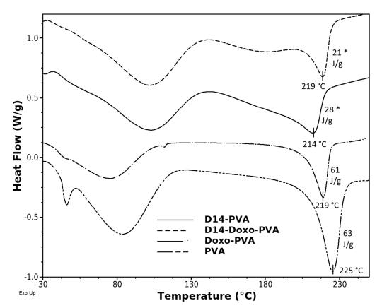
**Figure 3.** Differential scanning calorimetry thermograms of PVA spheres, D14-loaded PVA sphere, doxo-loaded PVA sphere and D14 and doxo-loaded PVA sphere. The y-axis represents watts/sample g (W/g). A statistically significant difference for D14 group is indicated by (\*).
