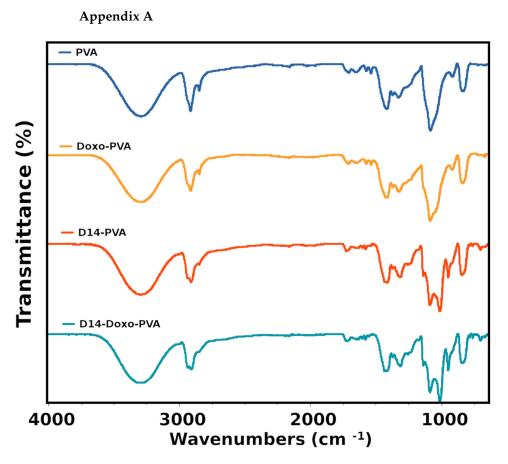
Figure A1. FTIR of the studied samples exhibiting the whole scanned region.
