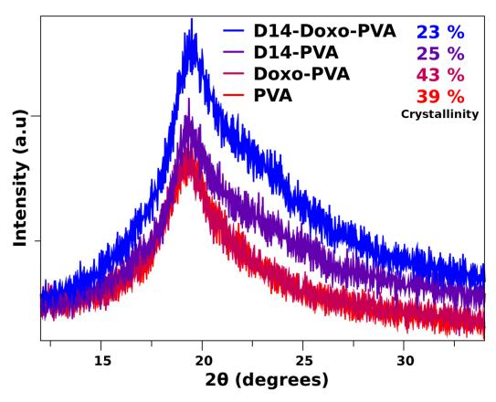
Figure 4. X-ray diffraction pattern of PVA sphere and loaded with D14, doxo and D14-Doxo.
