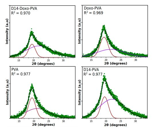
**Figure A4.** Deconvolution of the PVA majority peak into amorphous and crystallinity peaks in order to calculate the % crystallinity. Only two peaks were used for deconvolution in order to represent an average value of the whole hydrogel.
