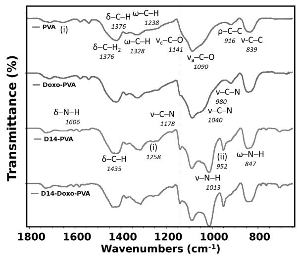
**Figure 2.** Fourier transform infrared spectroscopy (FTIR) analysis of PVA sphere, doxo-loaded PVA sphere, D14-loaded PVA sphere and D14 and doxo-loaded PVA sphere. In the figure, the symbols represent v—stretching,  $\delta$ —bending,  $\rho$ —rocking,  $\omega$ —wagging. Region (i) is water absorption and (ii) represents aromatic ketone—C-CO aryl skeletal vibration.
