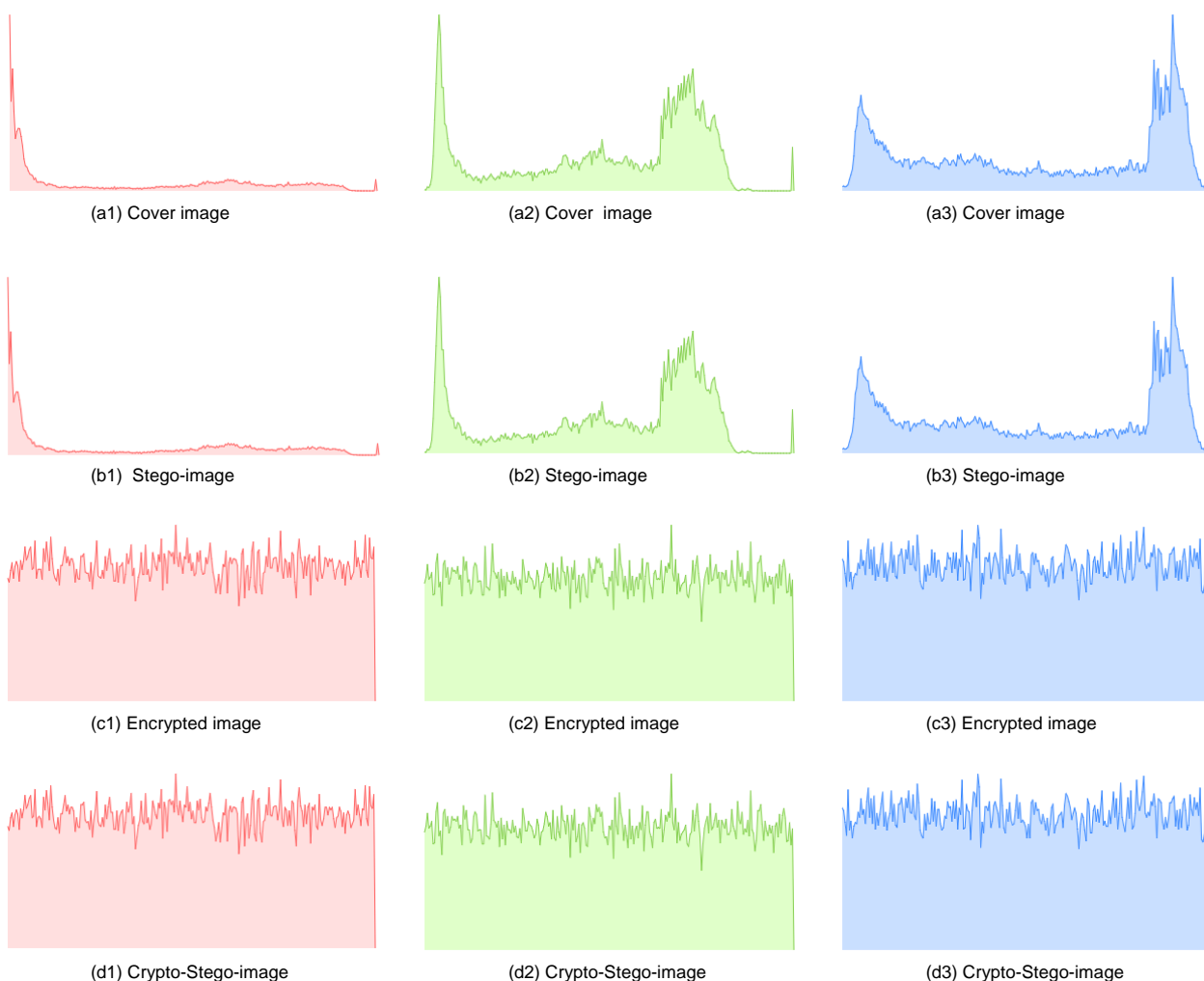
FIGURE 14. RGB Histograms of Profile image for R-, G- and B-channels: (a1, a2, a3) histogram of cover image, (b1, b2, b3) Histogram of stego-images, (c1, c2, c3) histogram of encrypted image, (d1, d2, d3) histogram of carrier image.
