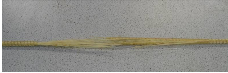
Figure 7: Ruptured GFRP during material test
