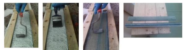
Figure 1. Hand lay-up: Images showing the rolling and wetting process; right, finished planks.
