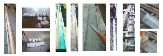
Figure 2. Left 9m long mould; 2<sup>nd</sup> left, 9m lengths of WR and SM prepared; 3<sup>rd</sup> left, mould coated with PVA release agent; left centre, finished plank; right centre, plank's rough edges being filled off; 3<sup>rd</sup> right, 5mm borings in flanges; 2<sup>nd</sup> right I-Beam with cleats glued and held to set using G-clamps; right, I-beams reinforced with woven rovings and shredded mat
