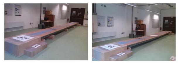
Figure 8. Left, footbridge set-up for rigid walking; right, flexible footbridge set-up
