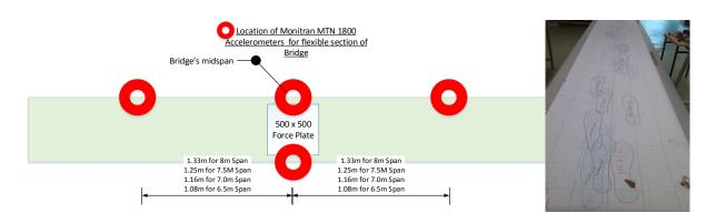
Figure 7: Left, location of accelerometers on bridge; right, grid paper ready to be measured
