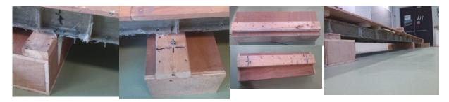
Figure 5. Left, pin connection for 8m span; centre left, opening and arrangement for pin connection for 6.5m to 7.5m spans; centre right, roller support top, and pin support bottom; right, rigid support arrangement
