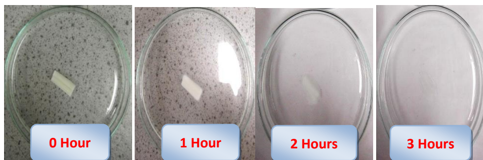
Figure-8. Degradation analysis of representative Batch A7 sample
