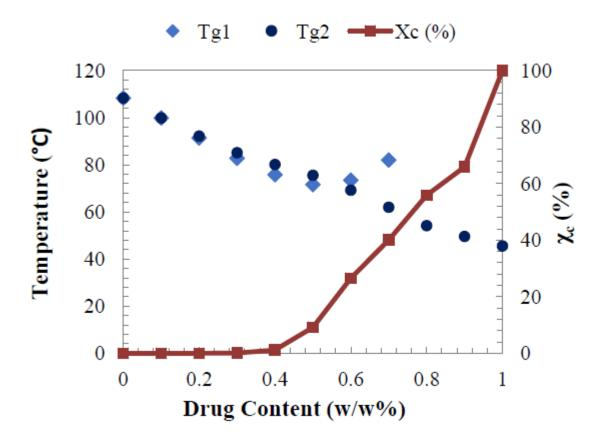
Figure 3: Gordon Taylor and Fox equations fit to the variation of the glass transition temperature of annealed physical mixtures of PVPVA and IND with the concentration.
