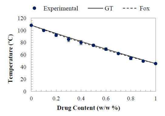
Figure 4: Glass transition temperature of annealed physical mixtures of PVPVA and IND as a function of the concentration. The points represent the experimental values; the line represents the BCKV fit.
