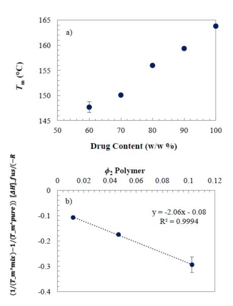
Figure 6: Polymer-drug interaction parameter as a function of temperature. The line represents the best fit of Equation 13 to experimental data.
