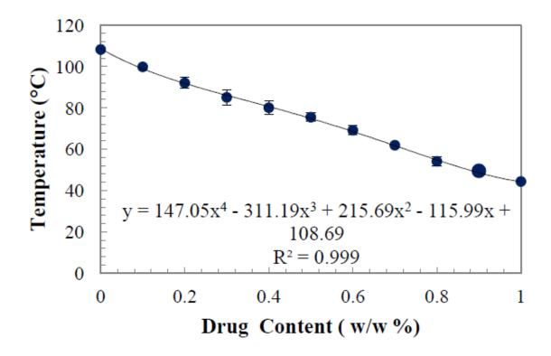
Figure 5: a) Melting temperature of IND as a function of its volume fraction. b) Plot used to determine the F-H interaction parameter of PVPVA-IND system close to the melting temperature of the drug.
