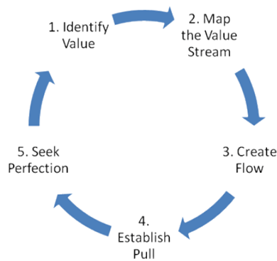
Figure 5: The continuous cycle of the Five principles of Lean Thinking (Womack and Jones 2003).
