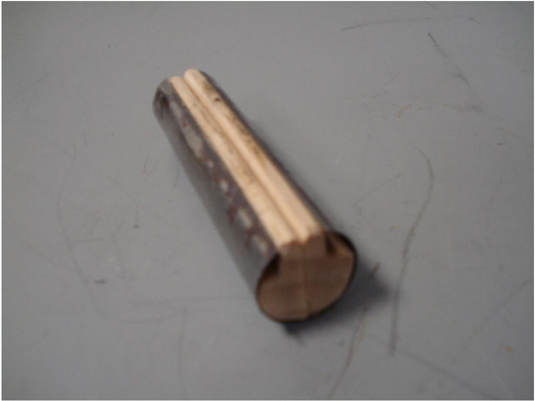
Figure D5 Centrifuge prototype geogrid restraint
