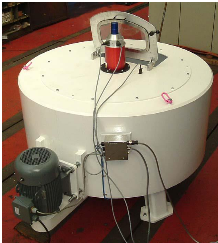
Figure 3.4 The IT Sligo 9g-tonne geotechnical centrifuge
