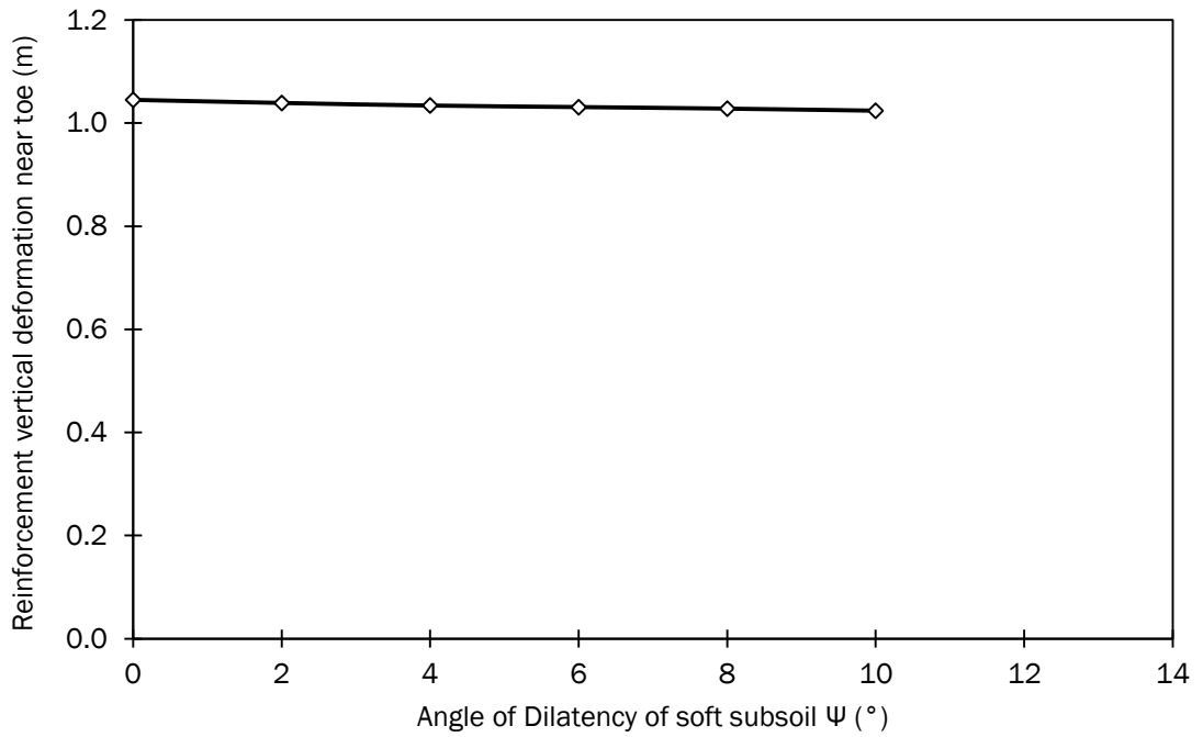
Figure A4 Vertical deformation of reinforcement near the embankment toe for a range of subsoil angle of dilatancy \Psi ( ^{\circ} )
