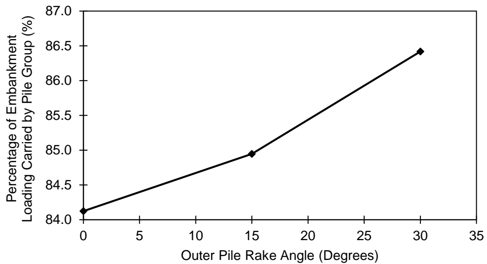
Figure 5.37 Pile group efficacy (%) for a range of outer pile rake angle (Degree (°)) ( H = 4.0m , J_{re} = 500kN/m and s = 3.0m )
