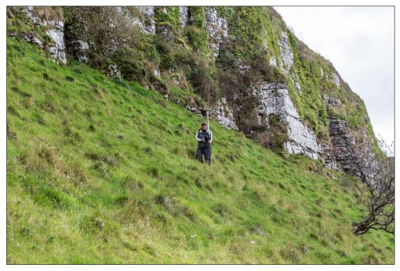
Figure 3.8: Slope measurements at the Keash Caves, Co. Sligo using RTK enabled GPS.
