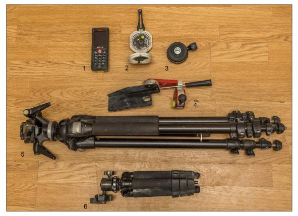
*Figure 3.7: Cave survey equipment: 1 - digital distance meter. 2 - compass. 3 - 360° panning base plate. 4 - instrument bracket. 5 - large tripod with 3D head. 6 - small tripod with ball head.*
