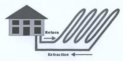
Fig. 3-5 Horizontal closed loop collector in series
