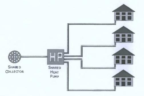
Fig. 4-1 District heating system with shared heat source and shared heat pump.
