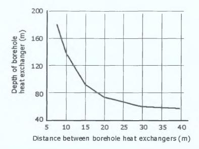
Fig. 3-9 Borehole spacing [Sanner, 2004]
