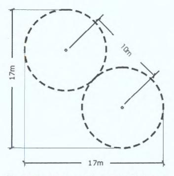
Fig. 5-2 Borehole spacing for individual collectors
