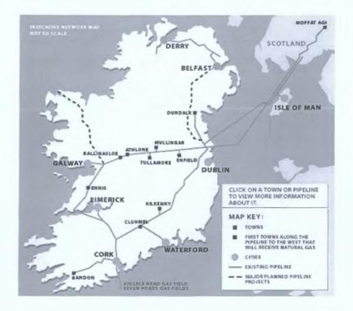
Fig. 3-10 Natural gas network in Ireland [Source: an Bord Gais]
