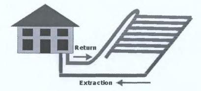
Fig. 3-6 Horizontal closed loop collector in parallel
