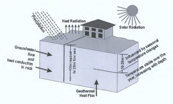
Fig. 3-2 Delivery and storage of heat energy in the ground [Sanner, 2002] There are a number of different forms of geothermal energy, many of which are particularly suited to Irish climate, geology and soils. The different forms are listed below.
