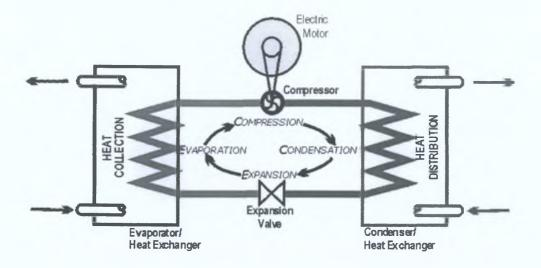
Fig. 3-3 How a heat pump works
