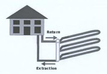
Fig. 3-7 Horizontal closed loop trench collector
