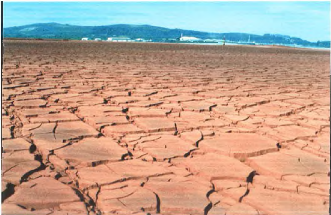
Plate 1.1. View of section of red mud stack showing mosaic cracking of surface
