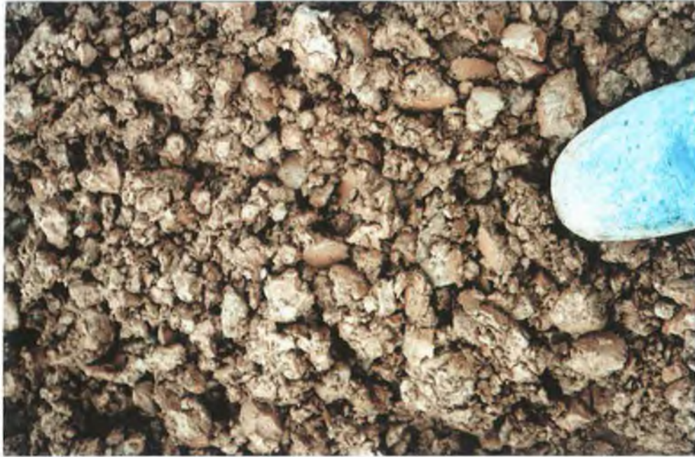
Plate 4.6. Mud Surface Following Addition of Process Sand and Gypsum
