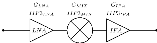
Fig. 3. RF front-end cascade: LNA, mixer and IF amplifier.
